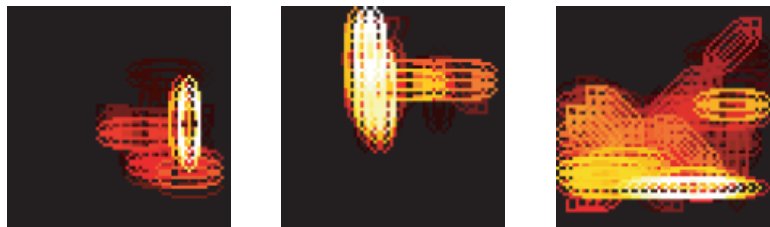
Figure 2.3: Example visualizations of prototypes taken from Serre et al. [6], corresponding to airplanes (left), faces (middle), and motorcycles (right). Here, an oval indicates the location and scale of an edge detector (i.e., an S1 unit), while color indicates the contrast of those edges.
